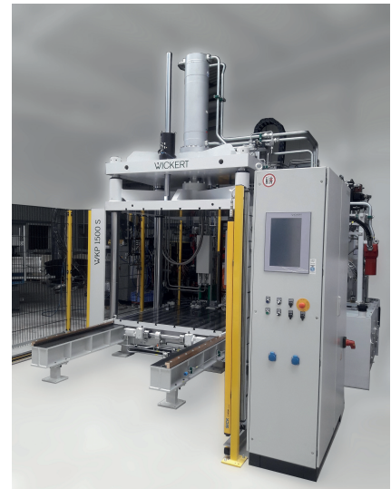
Fig. 4. Roof linings for passenger cars are produced on Wickert presses like this WKP 1500 S, in some cases also using composites which include natural fiber-reinforced plastics (NFRP) © Wickert
