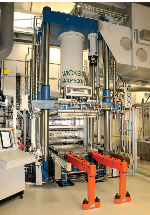
Fig. 3. Organo sheets are turned into 3D components at the research institute Neue Materialien Bayreuth (NMB): composite press for high-performance thermoplastics with processing temperatures of up to 450 °C
