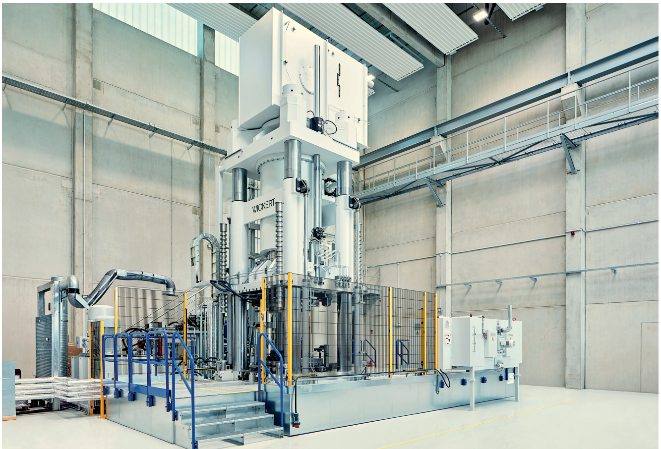
Composite press for research: for scientists at the Chemnitz University of Technology, Wickert developed a highly flexible four-column upper piston press which offers a high level of freedom and diversity in application © TU Chemnitz
